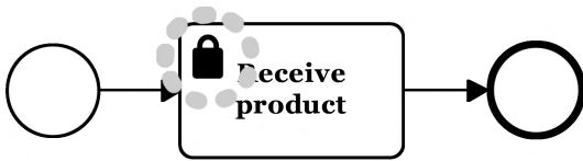
Figure 4: Example of annotation on modeling language elements, based on the proposal of Leitner et al. [56]: the augmentation of the process model element is made through the superposition of an icon (indicated by the dotted circle) to an activity and, in this case, represents that the augmented activity involves some kind of access permission.
